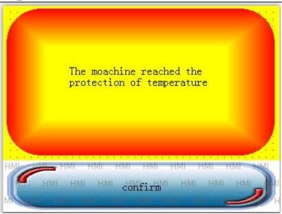
温度超过报警值, 按下面"CONFIRM"确认以消除报警 If temperature exceeds the alarm limit, you may press "Confirm" button to clear the alarm.
