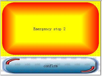
急停按钮 被按下, 按下面"CONFIRM"确认以消除报警 After emergency stop button is pressed, you may press "Confirm" button to clear the alarm.
