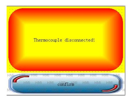
Thermocouple disconnected: please check all temperature thermocouple
